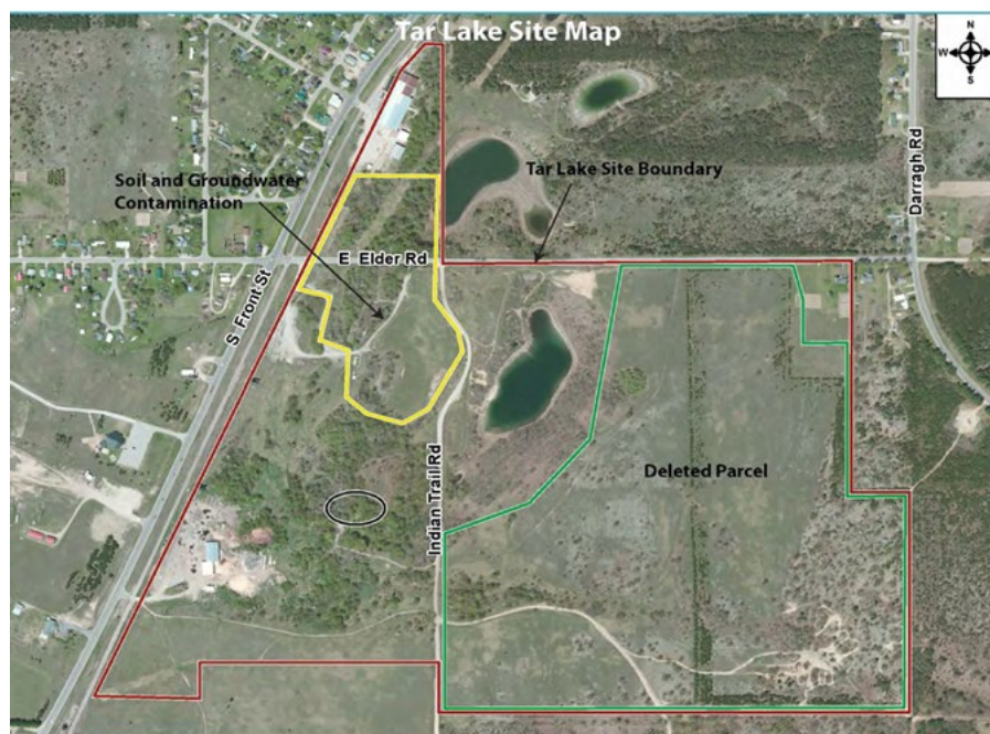
Figure 10. Map of Tar Lake Plume in Antrim County showing the site boundary, remediated portion (in green) and soil & groundwater contamination (in yellow). 293
