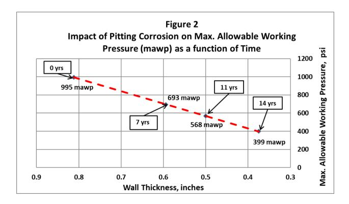
Figure 2 is a plot of Maximum Allowable Working Pressure (mawp) for schedule 60, 20 inch outside diameter, seamless carbon steel pipe. <sup>19</sup> This is the pipe that was installed at the Straits of Mackinac in 1953.
